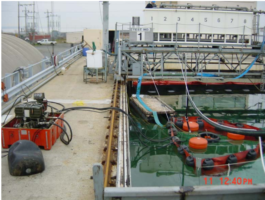
Figure 3. Photo showing power pack on deck, skimmer discharge hose to recovery tanks and inline mixer.
