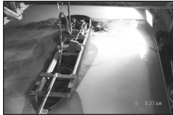
**Figure 6 Model working in level ice.**
